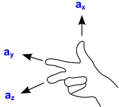
“right-hand rule“ for orientation of axis  $a_{x,y,z}$
